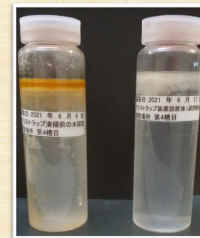
Water in grease trap 左 | O3ZF Before 右 | O3ZF After
